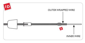
**5** Slide the outer wrapped wire back to expose the inner wire.
