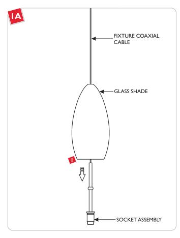
Feed the fixture coaxial cable through the glass shade. Slide the glass shade down the cord and rest it onto the socket assembly.
