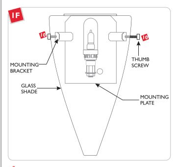
Place the glass shade onto the mounting plate. Align the glass shade holes with the mounting plate holes. Tighten the thumb screws to secure the glass shade in place.
