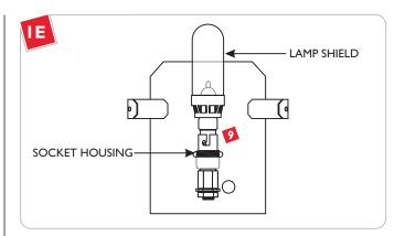
Place the lamp shield onto the socket housing. Screw
