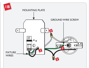
2 Feed the fixture wires through the mounting plate side hole.
