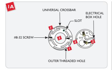
Make sure the two outer threaded holes on the universal crossbar are positioned at 45° degree diagonal, so that they match with the mounting bracket slotted holes.
