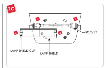
Install the lamp shield, by snapping the lamp shield clips onto the sockets.
