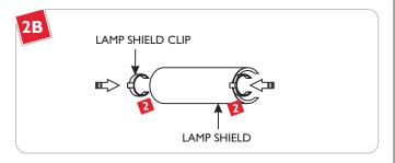
2 Snap the lamp shield clips onto the lamp shield ends.
