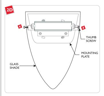
Place the glass shade onto the mounting plate. Align the glass shade holes with the mounting plate holes. Tighten the thumb screws to secure the glass shade in place.
