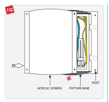
Replace the acrylic screen onto the fixture base. Make sure that the acrylic screen holes are properly set onto the fixture base posts. Hold the acrylic screen in place. **Omit this step for Stingray Venus.**
