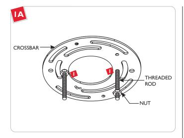
Screw one nut onto each threaded rod and tighten it to secure the threaded rod in place.
