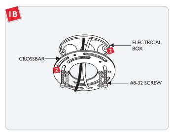
Mount the crossbar to the electrical box with two #8-32 screws.
