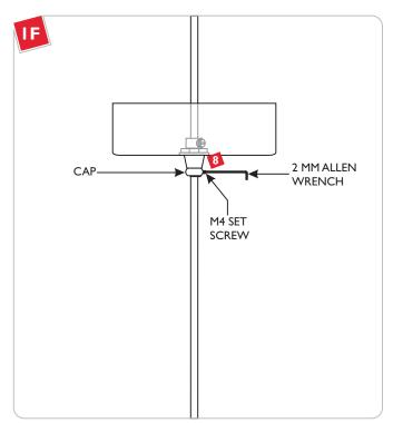
Slide the canopy up against the plastic strain relief and tighten the M4 set screw snugly on the cap with 2 MM Allen wrench.
