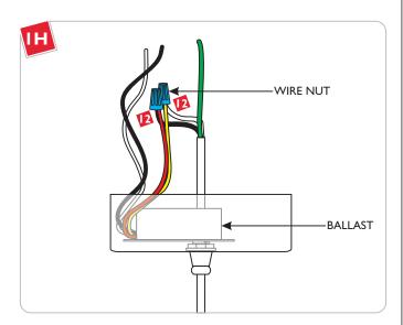
Connect one ballast wire to each fixture wire (except ground wire) with a wire nut.
