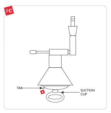
Remove the suction cup by pulling on the tab.
