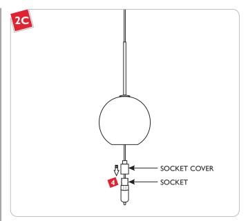
1 Lower the socket cover onto the socket.
