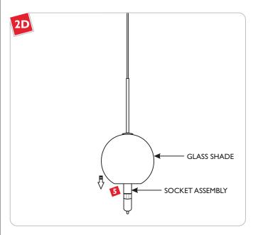
5 Lower the glass shade onto the socket assembly.
