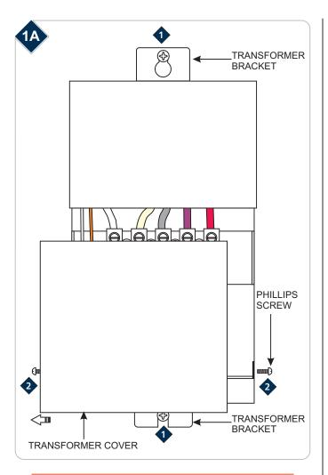
**NOTE:** In order to use small gage wires from the transformer to the electrical box, it is recommended to install the remote transformer near (if possible) the electrical box. See "Low Voltage Wire Size Table" below.
