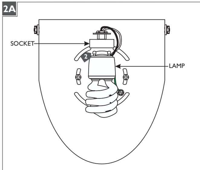
**CAUTION:** To reduce the risk of a burn or electric shock during relamping, disconnect the power to the fixture by turning the wall switch off.
