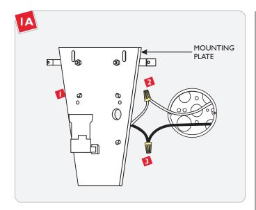
In accordance with local electrical codes, make sure that the mounting plate is grounded.
