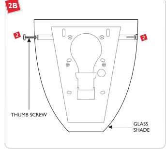
Place the glass shade onto the mounting plate. Align the glass shade holes with the mounting plate holes, replace and tighten the thumb screws to secure the glass shade in place.
