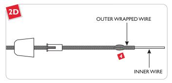
4 Slide the outer wrapped wire back to expose the inner wire.
