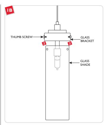
Place the glass shade completely into the glass bracket and tighten the three thumb screws to secure the glass shade in place.
