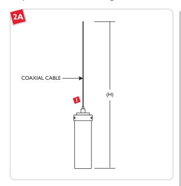
Cut the coaxial cable to the desired length with a sharp cutter. The overall fixture height (H) is measured from bottom of the glass shade to end of the coaxial cable.
