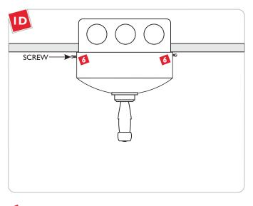
6 Reattach the dome cover to the backplate with the screws.
