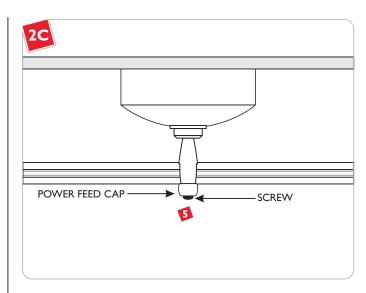
**5** Tighten the screw on the power feed cap for proper power connection.
