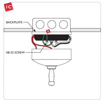
Mount the backplate to the electrical box with two #8-32 screws.
