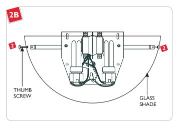
Place the glass shade onto the mounting plate. Align the glass shade holes with the mounting plate holes. Tighten the thumb screws to secure the glass shade in place.
