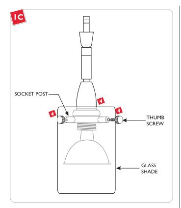
Align the glass shade holes with the socket posts. Tighten the three thumb screws to the bracket holes to secure the glass shade in place.
