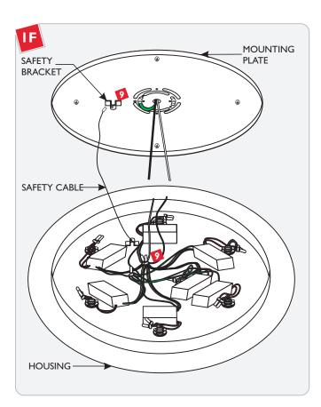
Insert one end of the safety cable into the mounting plate safety bracket and insert the other end into the housing safety bracket.
