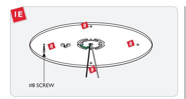
Secure the mounting plate to the anchors with the provided #8 screws.
