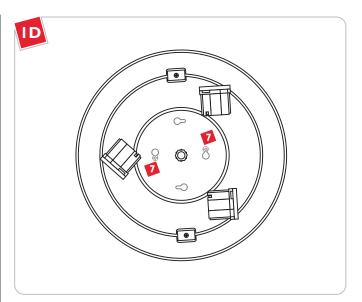
Rotate the mounting plate so that the #8-32 screw heads are locked into the small portion of the key holes.
