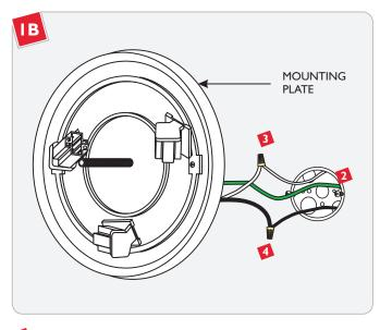
In accordance with local electrical codes, make sure that the fixture is grounded.
