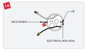
Thread (Not Completely) the two provided #8-32 screws into the electrical box holes, leaving 1/8" of them exposed.
