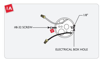
Thread (Not Completely) the two provided #8-32 screws into the electrical box holes, leaving 1/8" of them exposed.
