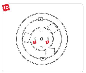
Rotate the mounting plate so that the #8-32 screw heads are locked into the small portion of the key holes.
