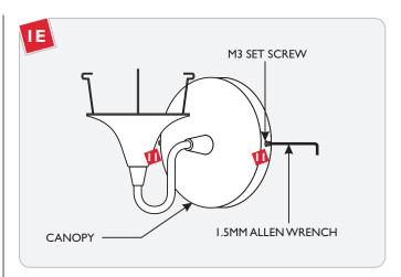
Place the fixture canopy onto the backplate. Level the fixture vertically and tighten the two M3 set screws with the I.5MM Allen wrench to secure the fixture in place.
