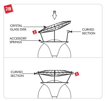
With the small hole section of the crystal glass disk facing towards lamp, place edge of the crystal glass disk into curved section of accessory springs.
