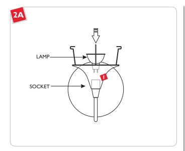
Use **MAX 35** Watt MRII Front Cover Halogen Lamp.
