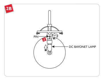
2 Push the lamp completely into the socket and rotate it clockwise to lock it in place.
