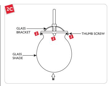
Place the glass shade completely into the glass bracket and tighten the three thumb screws to secure the glass shade in place.
