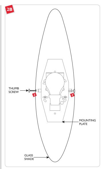
Place the glass shade onto the mounting plate. Align the glass shade holes with the mounting plate holes, replace and tighten the thumb screws to secure the glass shade in place.
