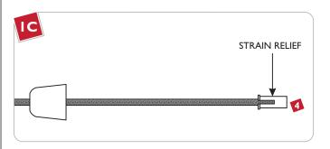
Insert the coaxial cable through the flared end of the strain relief.
