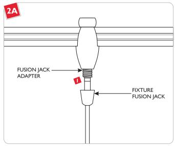
Push and screw the fixture Fusion Jack completely into the Fusion Jack adapter.
