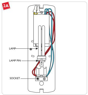
Use **MAX 18** Watt Type Quad Tube G24q-2 Base Compact Fluorescent.
