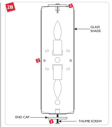
2 Place the glass shade onto the mounting plate.
