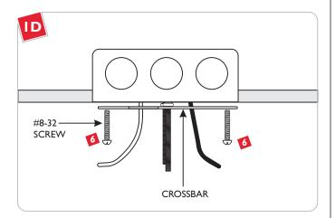
Install the crossbar to the electrical box with the two provided #8-32 screws.
