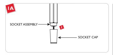
Unscrew and remove the socket cap from the socket assembly.
