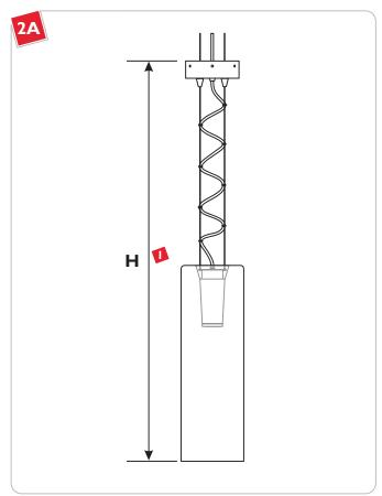
The overall fixture height (H) is measured from bottom of the glass shade to top of the canopy.
