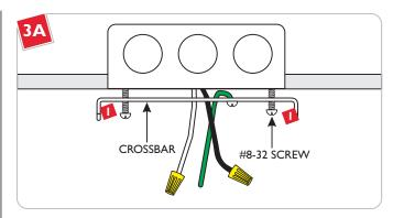
Mount the crossbar to the electrical box with the provided two #8-32 screws.
