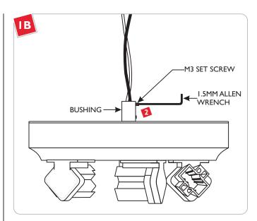
Loosen (Do Not Remove) the top M3 set screw on the bushing with the provided I.5MM Allen wrench.
