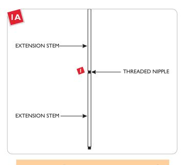
**NOTE:** Use a 24" extension stem for the minimum 32" overall height. To extend the fixture height to 44", or 56", or 68", use the additional 12", or 24", or combination of 12" and 24" provided extension stems respectively. The extension stems are not field cuttable.
