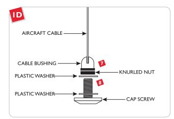
Remove the cap screw from the cable bushing.
