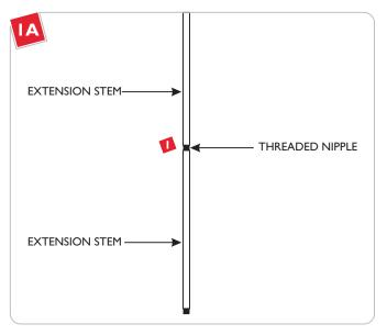
**NOTE:** Use a 24" stem for the minimum 32" overall height. To extend the fixture height to 44", or 56", or 68", use the additional 12", or 24", or combination of 12" and 24" provided extension stems respectively. The extension stems are not field cuttable.
