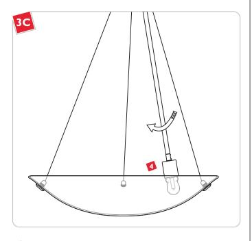
Carefully swing the socket assembly back into the glass shade.
