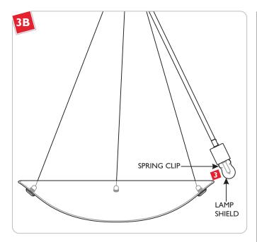
9 Push the lamp shield completely onto the socket spring clips.
