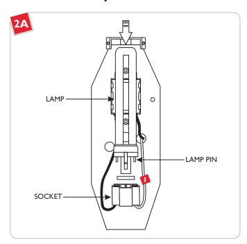
Use **MAX 9** Watt Type Twin Tube GX23 Base Compact Fluorescent Lamp.
