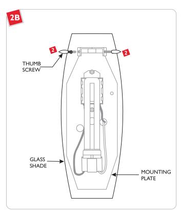
Place the glass shade onto the mounting plate. Align the glass shade holes with the mounting plate holes. Tighten the thumb screws to secure the glass shade in place.
