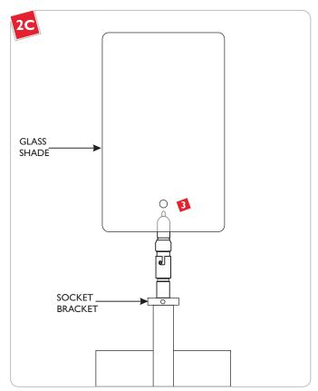
3 Align the glass shade holes with the socket bracket holes.
