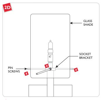
Tighten the four pin screws to secure the glass shade in place.
