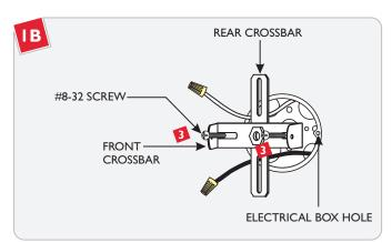
**NOTE:** To mount the crossbar assembly, use the front crossbar, with the electrical box containing a plaster ring, or use the rear crossbar, with the octagon electrical box.
