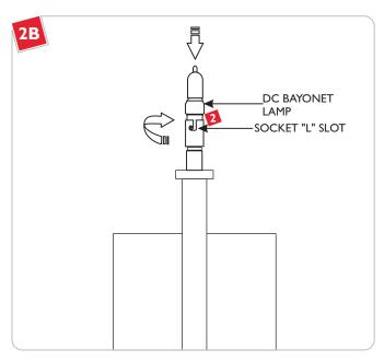
Push the lamp completely into the socket and rotate it clockwise to lock it in place.
