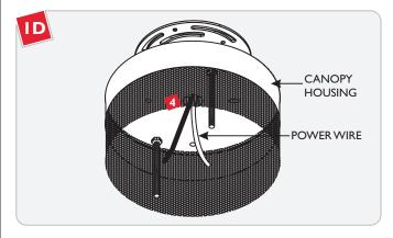
4 Feed the power wires through the canopy housing center hole.
