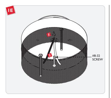
Align the canopy housing holes to the crossbar threaded holes and completely tighten the two provided #8-32 screws to secure the canopy housing in place.
