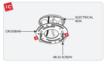
Mount the crossbar to the electrical box with the two #8-32 screws.
