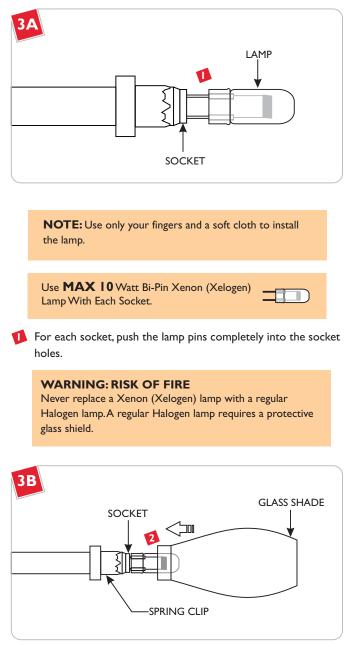
2 Push the glass shade completely onto the spring clip.
