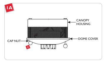
Remove the two cap nuts on the dome cover.
