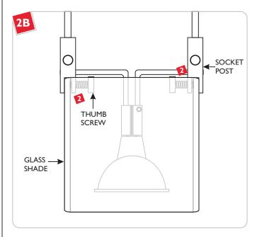
2 Slide the glass shade up into the socket post and secure it in place by tightening the two thumb screws.
