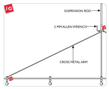
Hook one end of the cross metal arm to the socket post and hook the other end to the suspension rod post. Tighten the M4 set screw on the suspension rod post with the provided 2mm Allen wrench. Repeat this step for the other cross metal arm.
