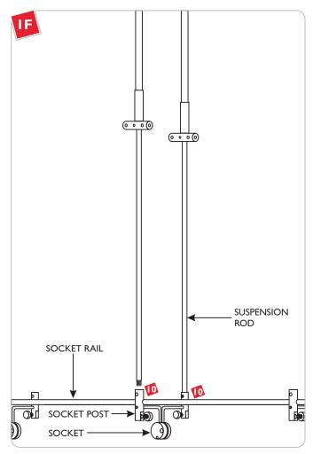
Screw the two suspension rods completely into the socket posts.
