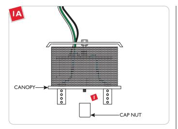
Remove the cap nut completely from the canopy.
