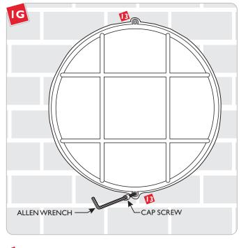
Replace the shade and tighten the cap screws to secure the shade to the fixture.
