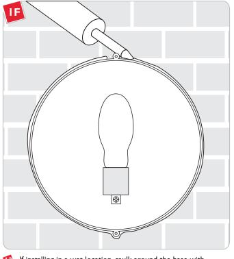
If installing in a wet location, caulk around the base with waterproof construction sealant.
