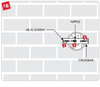
Attach the crossbar to the electrical box using the two #8-32 screws provided.
