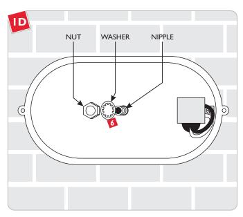
Make sure the fixture is level, and secure the fixture to the nipple with a lock washer and nut.
