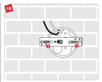
Attach the crossbar with nipple to the electrical box using two #8-32 screws provided.
