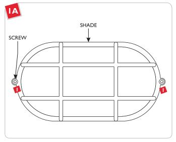
Remove the screws from the front of the fixture and remove the shade.
