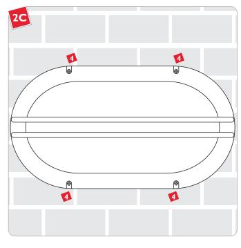
Replace the shade and reattach the screws to secure the shade to the fixture.
