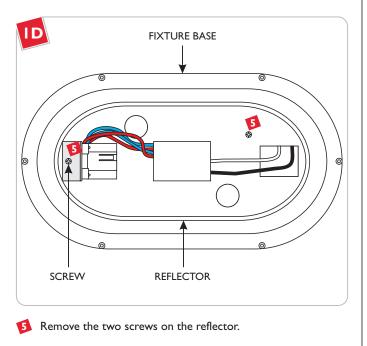
6 Lift the reflector out of the fixture base.
