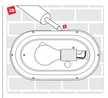
If installing in a wet location, caulk around the base with waterproof construction sealant.
