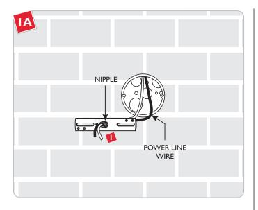
**1** Feed the power line wires through the crossbar nipple.
