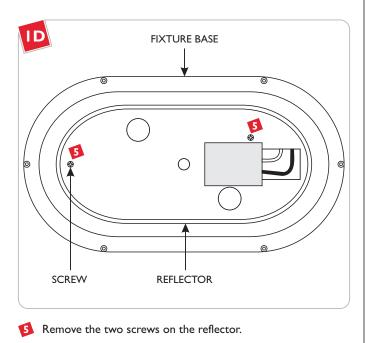
Lift the reflector out of the fixture base.
