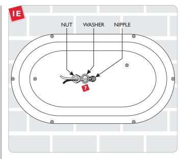
Make sure the fixture is level, and secure the fixture to the nipple with a lock washer and nut.
