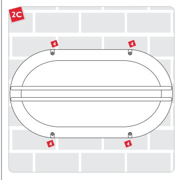
Replace the shade and reattach the screws to secure the shade to the fixture.
