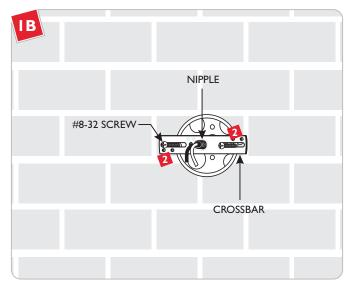
Attach the crossbar to the electrical box using two #8-32 screws provided.
