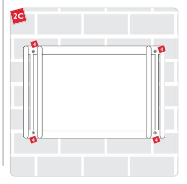
Replace the cover and reattach the screws to secure the cover to the fixture.
