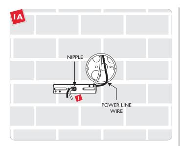
Feed the power line wires through the crossbar nipple.
