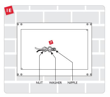
Make sure the fixture base is level, and secure it to the nipple with a lock washer and nut.
