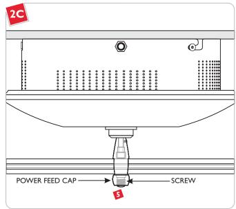
**1** Tighten the screw on the power feed cap for proper power connection.
