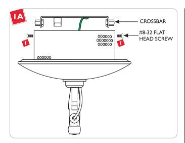
Remove the two #8-32 flat head screws to remove the crossbar.
