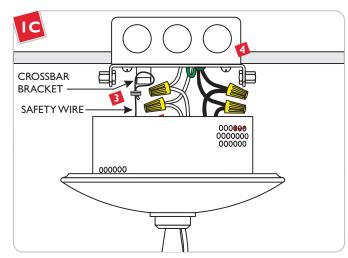
**NOTE:** All transformer power line wires must be connected to the same phase.
