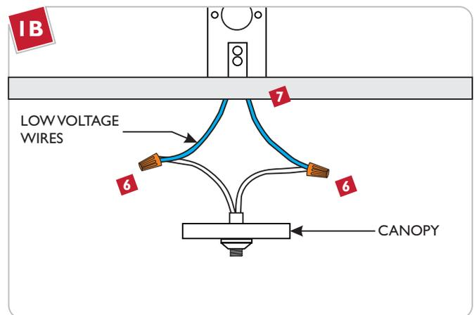
**NOTE:** The 2" electrical box must be installed prior to these steps. Refer to the instruction sheet provided with the electrical box.
