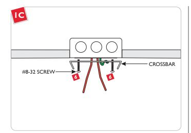
Mount the crossbar to the electrical box with the two #8-32 screws.
