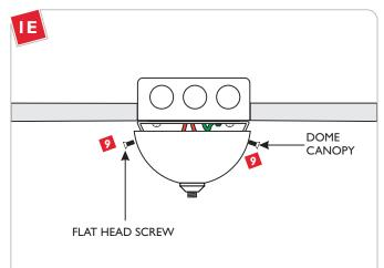
Line up the dome canopy holes with the crossbar holes. Replace and tighten the flat head screws to secure the dome canopy in place.
