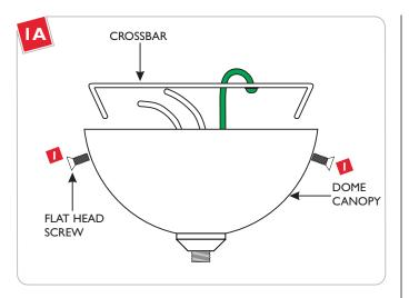
Loosen the two flat head screws to remove the crossbar from the dome canopy.
