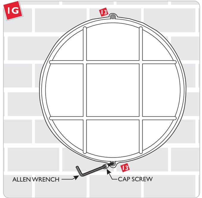
**1G** Replace the shade and tighten the cap screws to secure the shade to the fixture.
