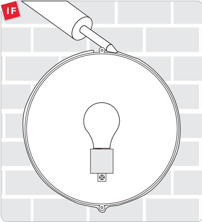
**1F** If installing in a wet location, caulk around the base with waterproof construction sealant.
