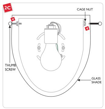
Tighten the thumb screws through the glass shade holes into the cage nut holes.
