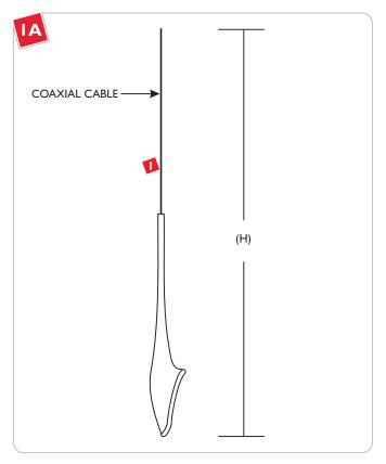
Cut the coaxial cable to the desired length with a sharp cutter. The overall fixture height (H) is measured from bottom of the glass shade to end of the coaxial cable.
