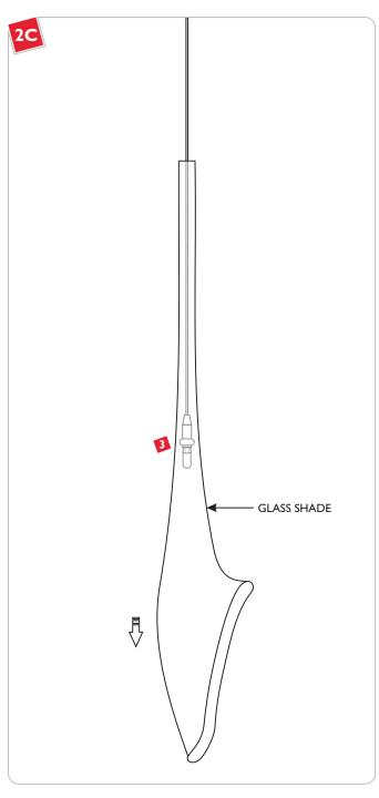
3 Lower the glass shade onto the socket assembly.
