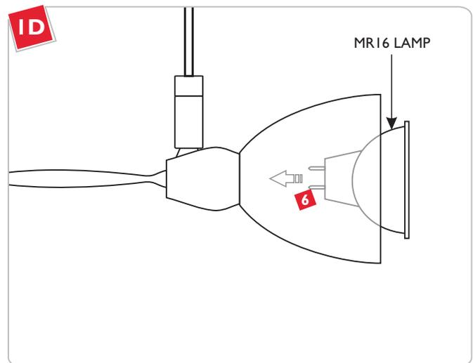
**6** Push the lamp pins all the way into the socket holes.
