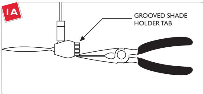
**1** If the Monty accessory fits tight onto the fixture, then carefully bend the grooved shade holder tabs in slightly with the needle-nose pliers. If it fits loose, then carefully bend the grooved shade holder tabs out slightly with the needle-nose pliers.
