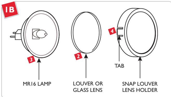
Use MAX 50Watt MR16 Front Cover Halogen Lamp.
