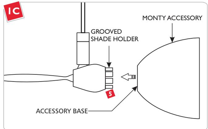
**5** Push the Monty accessory base onto the grooved shade holder.
