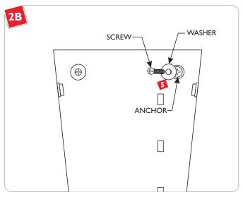
Slide a #8 screw through a washer and screw it into an anchor.
