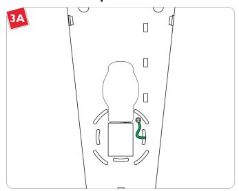
Use **MAX** 120 Volt, **60 Watt** Type BT15 Medium Base Lamp.
