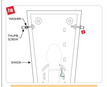
**NOTE:** Do not over tighten the thumb screws.
