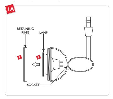
**CAUTION:** To reduce the risk of a burn or electric shock during relamping, disconnect the power to the fixture.
