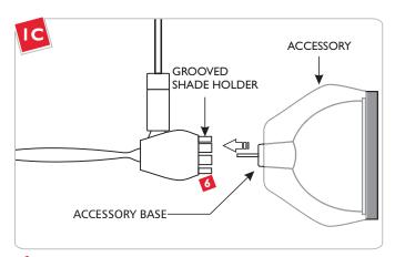
5 Line up the lamp pins with the socket holes.
