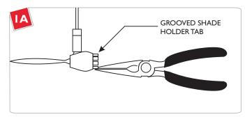
If the accessory fits tight onto the fixture, then carefully bend the grooved shade holder tabs in slightly with the needlenose pliers. If it fits loose, then carefully bend the grooved shade holder tabs out slightly with the needlenose pliers.
