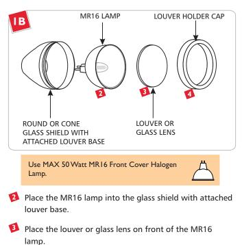
Screw the louver holder cap completely onto the louver base.
