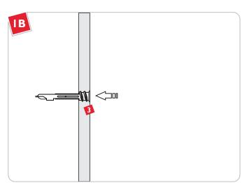
3 Screw the anchor in the rest of the way with a Phillips screwdriver.
