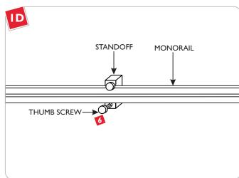
Place the MonoRail into the standoff slot. Use the thumb screws to secure the MonoRail to the standoffs.
