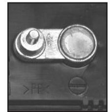
NEGATIVE POST HAS SMALLER DIAMETER
